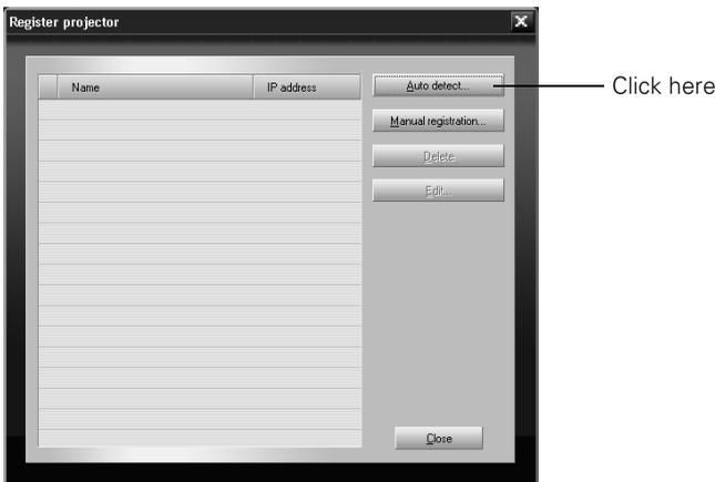
3. Click Auto detect to locate projectors currently operating on the network. Or click Manual registration and enter the projector's network IP address.
