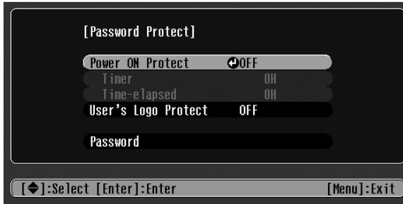
2. Use the
